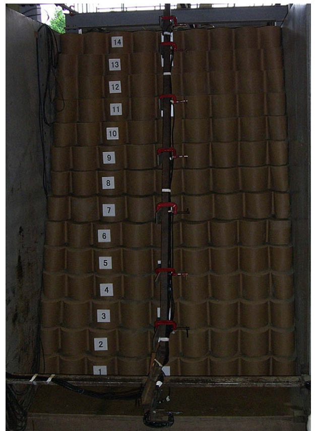
Fig. 11. Frontal view of wall in Test 3: post earthquake (159% of Kobe's PGA) – see excavated section of same wall in Fig. 3.
