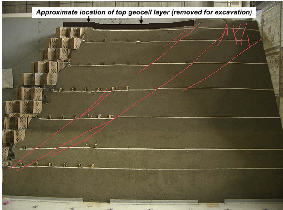
Fig. 9. Excavated section: Test 5 (PGA = 205% of Kobe's).
